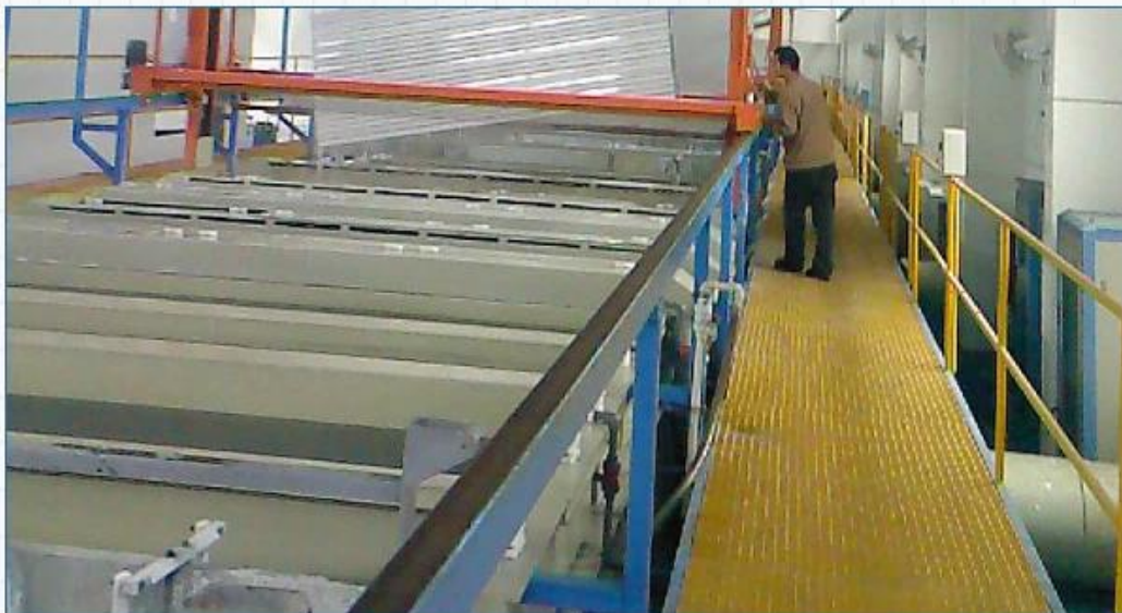
Aluminum profile anodizing line
