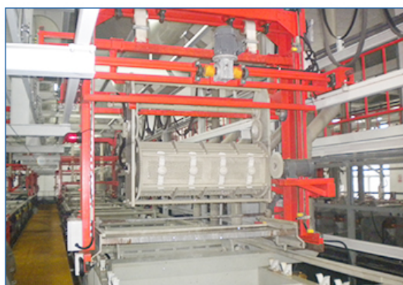
Nickel barrel plating line
