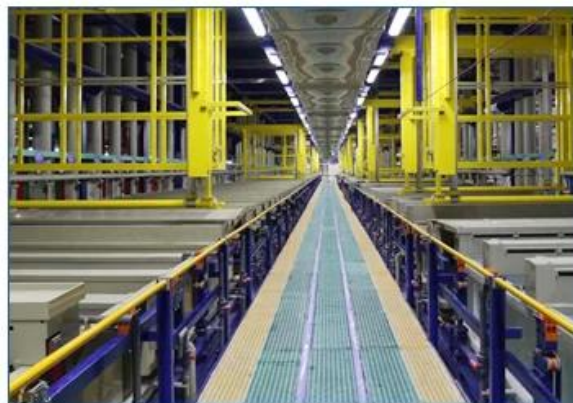
zinc electroplating line
