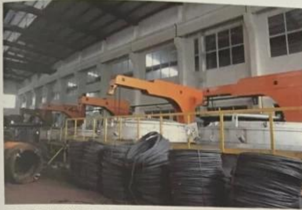
用于标准件行业球化炉 Used for fastner industry
