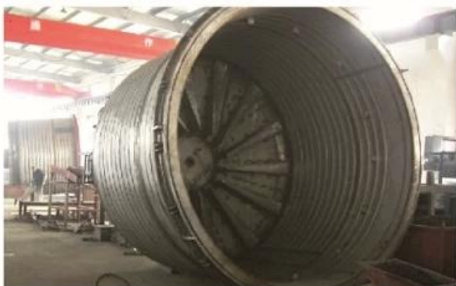
Liner of Well Type Electric Annealing Furnace
