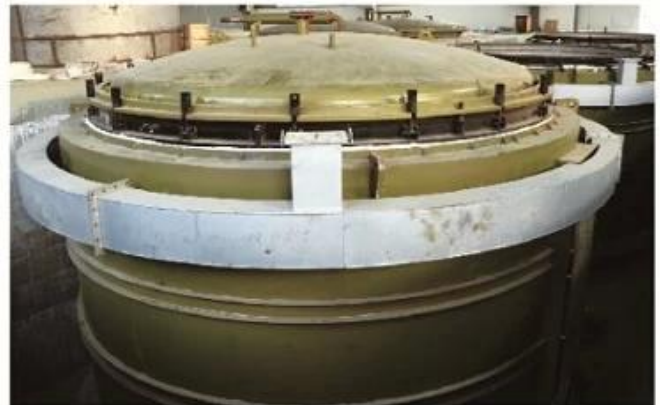
Well Type Electric Annealing Furnace (Main Furnace)
