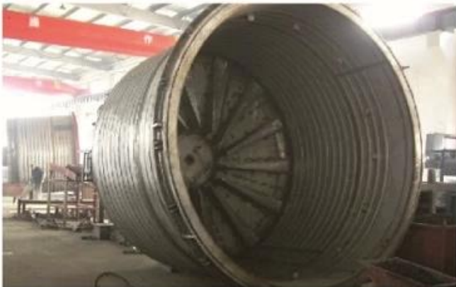
Liner of Well Type Electric Annealing Furnace
