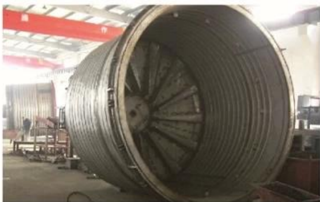
Liner of Well Type Electric Annealing Furnace
