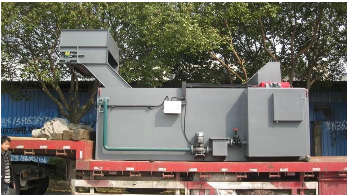
Quenching oil TANK:
