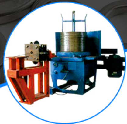
Belt wire drawing machine
