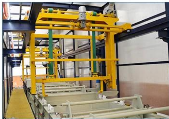
Zinc barrel plating line
