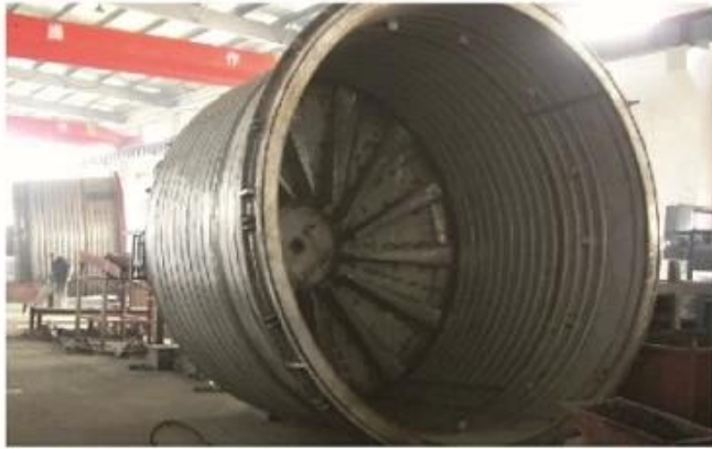
Liner of Well Type Electric Annealing Furnace
