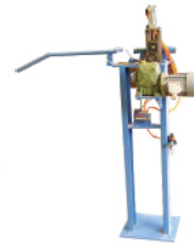
3-5mm- 6mm- 8-10mm Coil Collection Machine
