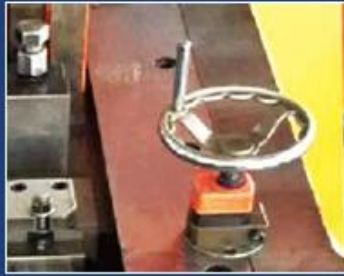
DIGITAL BAFFLING OPERATED BY HAND WHEEL
