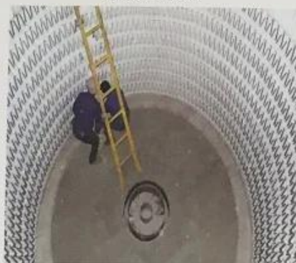
电加热炉 Electric heating furnace
