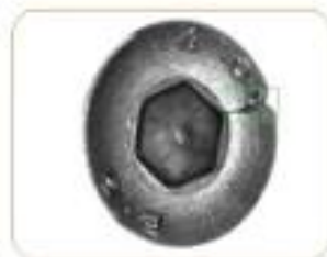
头部破裂 The head broken
