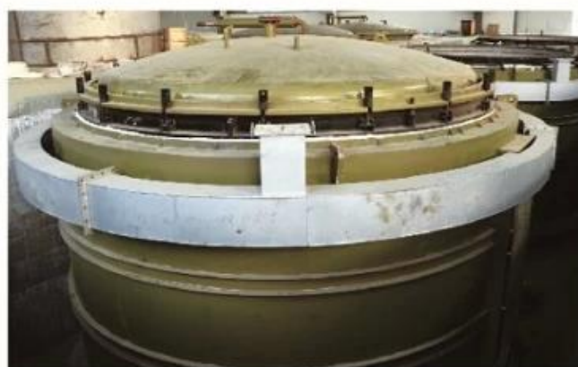
Well Type Electric Annealing Furnace (Main Furnace)
