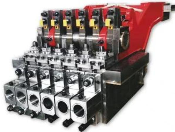
High accuracy main sliding block is designed to be connected with rear wing for letting it run stably and precisely, the bottom of front and back wing is adopted super wearing inserted copper plate with self lubrication, it can ensure accuracy and extend service life. The post stations of punching tool can be fulfilled the function of reverse punching.
