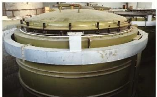
Well Type Electric Annealing Furnace (Main Furnace)
