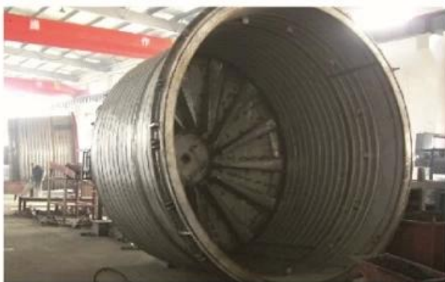
Liner of Well Type Electric Annealing Furnace
