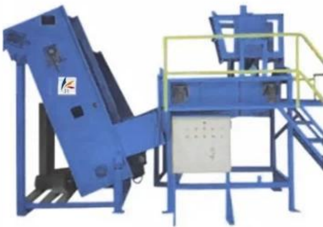
MAGNETIC-BELT TYPE FEEDER
