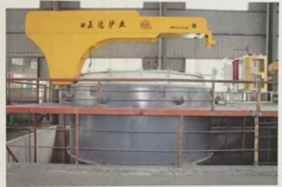
用于轴承行业球化炉 Used for the bearing industry
