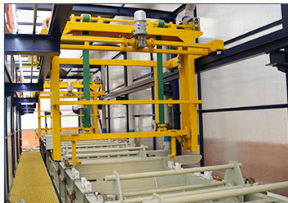
Zinc barrel plating line
