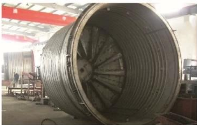
Liner of Well Type Electric Annealing Furnace
