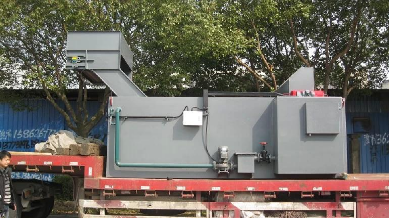
Quenching oil TANK:
