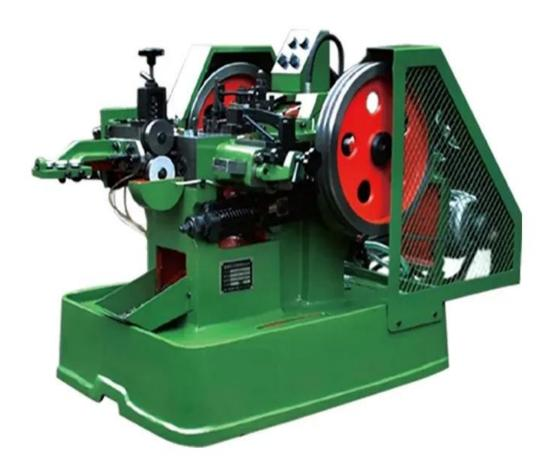
The heading machine is professional cold upsetting forming machine, which is matched with automatic thread rolling machine in the whole plant of m aking screws.
