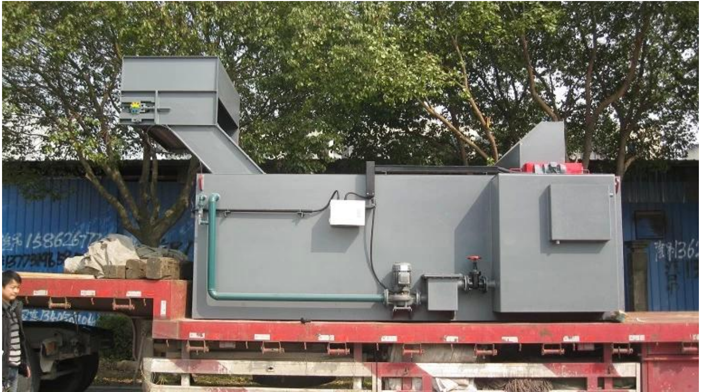
Quenching oil TANK:
