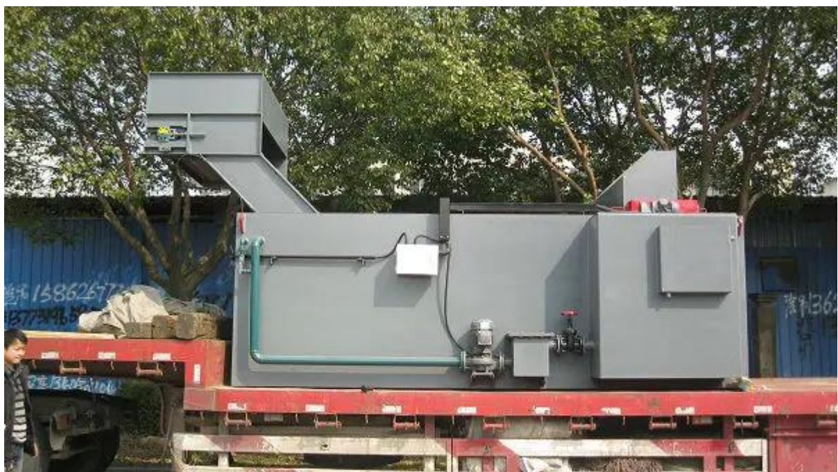
QUENCHIN OOLING TANK:
