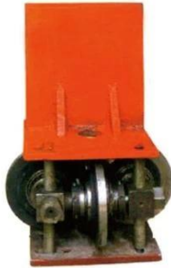
Die for Belt Wire Drawing
