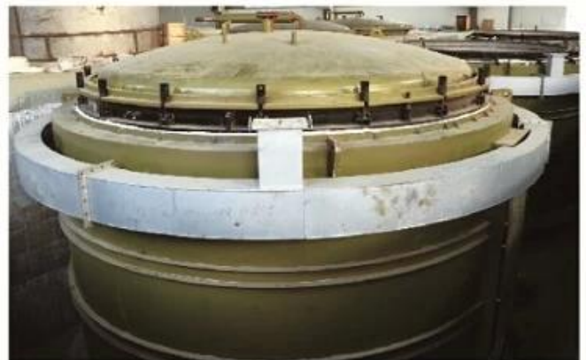
Well Type Electric Annealing Furnace (Main Furnace)
