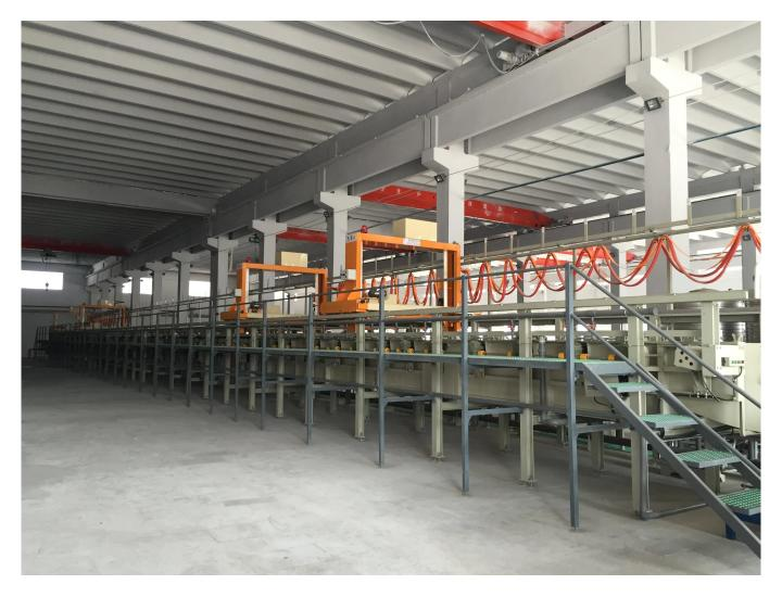
Barrel plating automatic production line can be adapted to a variety of small parts, standard parts and various types of plating needs substantial increase in labor productivity. Plating has been provided to expect from the rejection of the full set of water and drying equipment.
