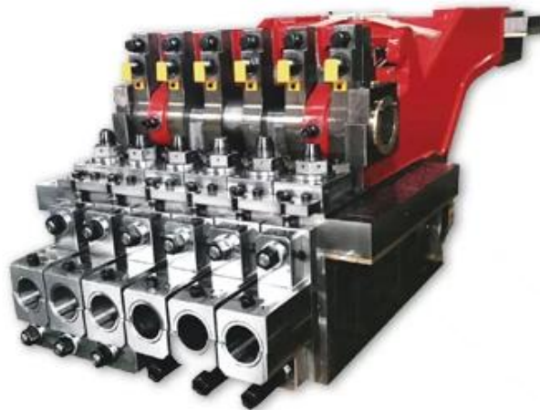
THE SWING OF GRIPPER IS DRIVEN BY CONJUGATE CAM
