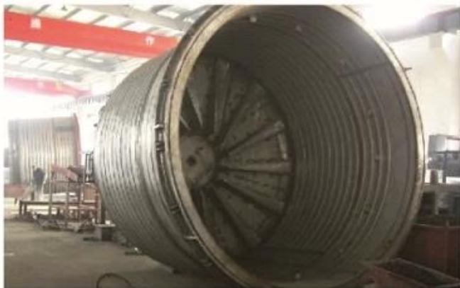
Liner of Well Type Electric Annealing Furnace
