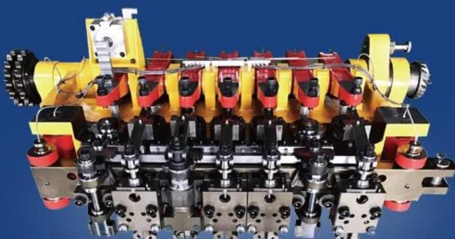
Due to the high accurate multi-function compound gripping mechanism, there are translational wide open gripper, nut gripper and turnover wide open gripper, and these 3 grippers can be interchanged and shared at will. However the key breakthrough design is that the turnover wide open gripper can both turn over and widely open, it expands the production range for different kinds of abnormal parts and reduces the manufacturing cost for the dies.
