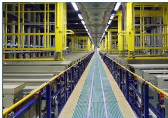
zinc electroplating line
