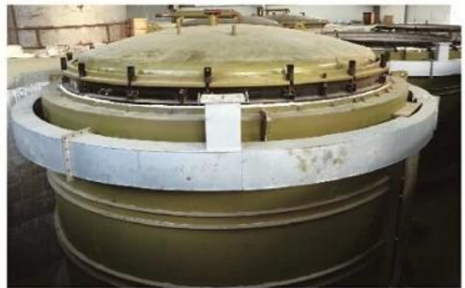
Well Type Electric Annealing Furnace (Main Furnace)
