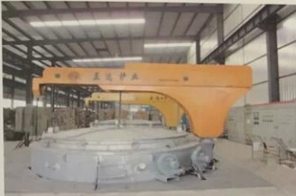
用于五金工具行业球化炉 Used for the hardware tool industry
