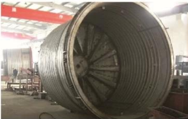
Liner of Well Type Electric Annealing Furnace
