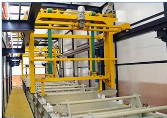
Zinc barrel plating line
