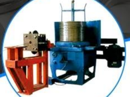
Belt wire drawing machine
