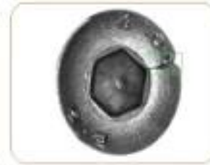
头部破裂 The head broken
