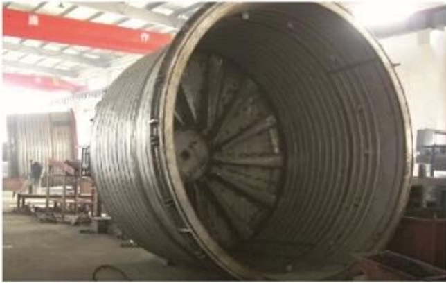
Liner of Well Type Electric Annealing Furnace
