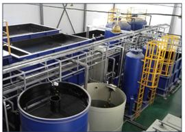
The exhaust gas treatment system mainly includes the suction hood \ suction pipe \ FRP fan, the exhaust gas treatment tower, the circulating pump, the tank and the pipeline. Mainly involved in the production of electroplating production of various types of chromium emissions, cyanide gas, acid waste gas, alkali waste gas and other comprehensive waste gas. After discharge standards.
